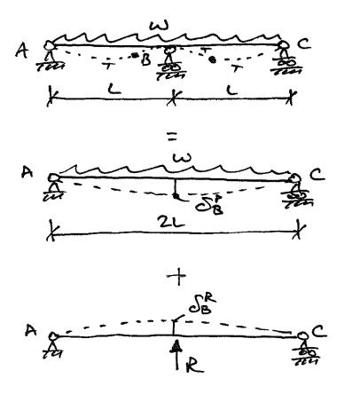
Once again we use compatibility of displacements for the original structure to write:
