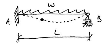
Using superposition we can break it up as follows (i.e. we choose a redundant):
