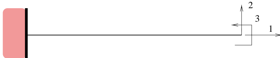
(b) : Structural Model for Cantilever Beam
