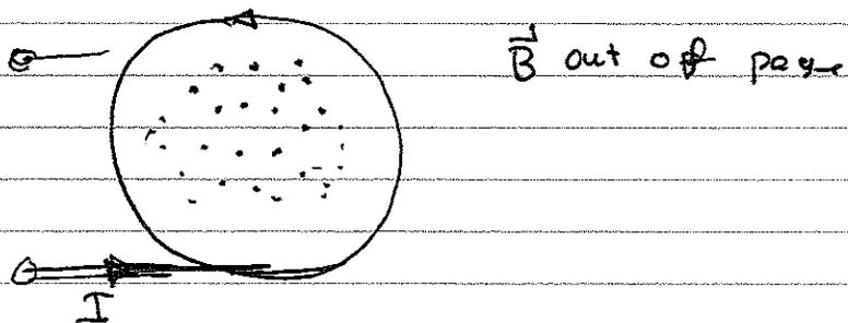
Calculate induced  $\vec{E}$ -field as a function of  $r$
