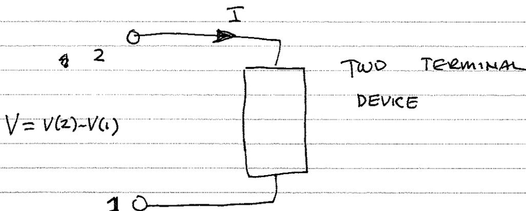
Using the electrical engineering convention, the power delivered to a 2-terminal device is
