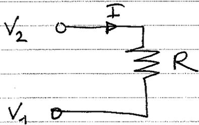
$$V_R = (V_2 - V_1) = IR$$
