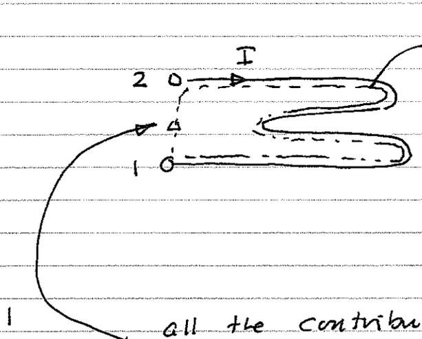
most of dotted loop is parallel to a good conductor.  $\vec{E} \cdot d\vec{s} = 0$
