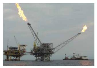
Figure 3. Other multi-point flare systems are elevated.
