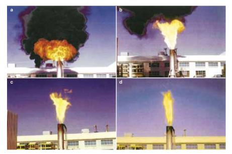
▲ Figure 9. Air assist is effective at smoke suppression: (a) no blower air; (b) blower is started; (c) air flow is increasing; (d) smokeless burning. Image courtesy of CRC Press (7).
