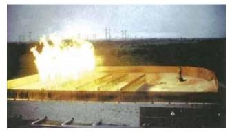
▲ Figure 2. Some multi-point flare systems are located at or near grade. Image courtesy of CRC Press (7).
