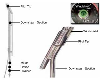
▲ Figure 11. Pilots consist of a mixer or venturi, a gas orifice, a downstream section that connects the mixer and the tip, and a tip.
